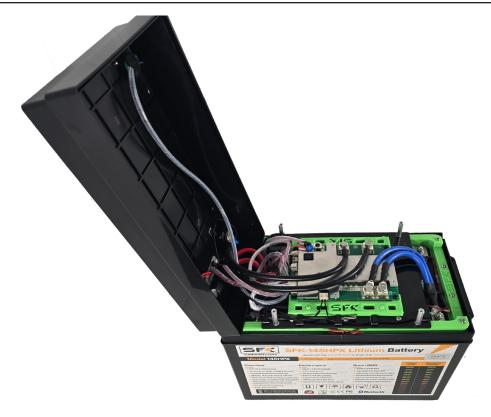
We only recommend opening the lid of your battery with hand tools and not with powered screwdrivers or impact drivers. Only use insulated tools when working with the battery with its lid open.
