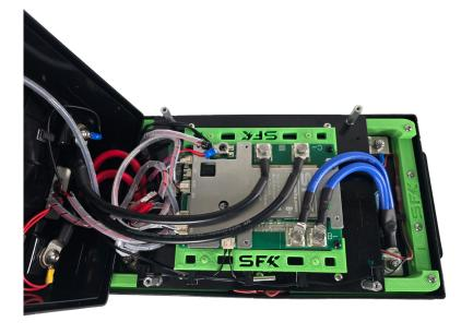
Ensure the wires are tight and make good contact with components, tighten if needed.
